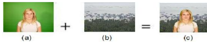
Gambar 1. Efek Chroma Key (a) foreground frame (b) background frame (c) frame hasil
